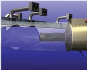
**B.** Small vinyl polymer aerosol particles are kept suspended in the airflow by a continuous air movement.
